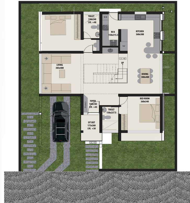
GROUND FLOOR PLAN AREA- 146.13m2(1572Sq.ft) FIRST FLOOR PLAN AREA- 110.85m2(1193Sq.ft) TOTAL- 256.98m2(2765Sq.ft)
